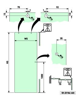
Only make the 10 mm glass drill hole if using the Aquant handle.
