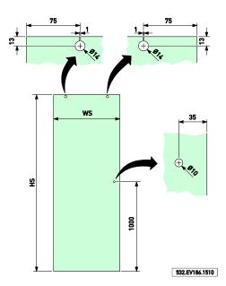
Only make the 10 mm glass drill hole if using the Aquant handle.
