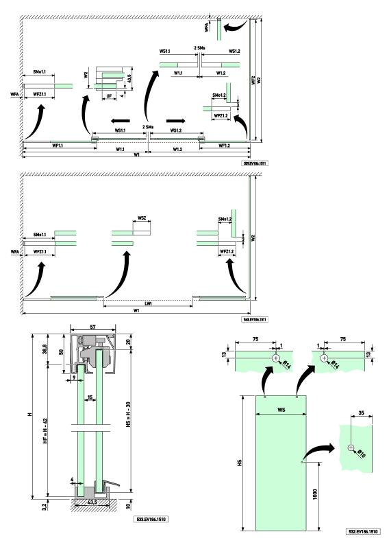
Only make the 10 mm glass drill hole if using the Aquant handle.
