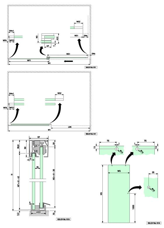
Only make the 10 mm glass drill hole if using the Aquant handle.  $\,$
